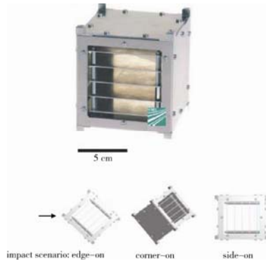
图 15 撞击靶结构及不同弹丸撞击方向 Fig. 15 Target structure and the different impact directions of projectile
