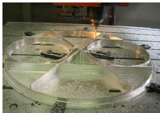
图6 实现整体加工的大型镁合金结构件 Fig. 6 Large-scale Mg alloy structure part made by machining as a whole
