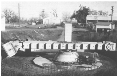
图 4-47 Davis 离心机第一阶段在露天地坑中转起来 Fig. 4-47 The Davis centrifuge first stage operating in the outdoor pit
