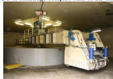
图 4-50 Davis 离心机复合振动台状态之二 Fig. 4-50 Davis centrifuge complex state of the shaking table II
