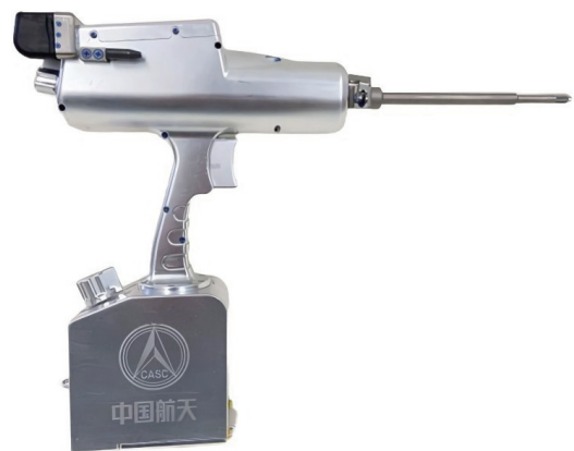
图1 中国空间站舱外电动工具实物 Fig. 1 Photo of extravehicular power tool used for China's Space Station
