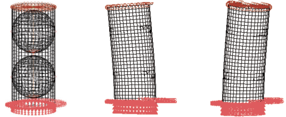
图 19 贮箱串联布局承力筒结构有限元模型及模态振型 Fig. 19 Finite element model and modal vibration mode of the serial layout load-bearing cylinder structure of the storage tank
