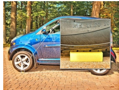
图 7 聚合物气凝胶对抗汽车压力的情况 Fig. 7 Smart car parked on top of a thick piece of polymer aerogel
