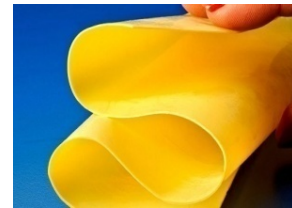
图 8 薄片聚合物气凝胶的实物照片 Fig. 8 Flexible sheets of NASA's new polymer aerogel
